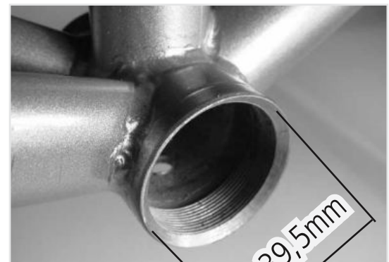
Fig. 3: Correct diameter of chamfering is most important for perfect function!
