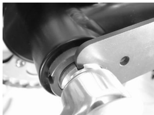
Fig. 8: Adjusting of gearing play. No preload!
