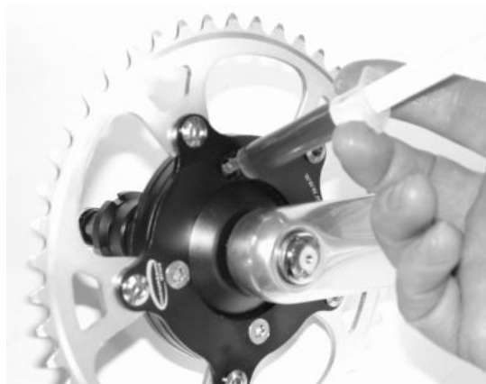
Fig. 7: Lubrication. insert about 1/3 of the syringe once or twice a year.
